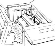
**6** Swing the printer cover back down. Push down on a portion of the cover to lock the cover into its normal position.
